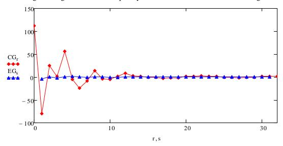
It is seen that the decay of the frequency coefficients is rapid for the DCT (i.e. CG<sub>r</sub>) but it is far outperformed by the EDFT.
